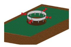
Position the ring over the top of the hole and insert the ring slowly, at this stage the Tree Ring will still be flexible which will allow you to adjust the ring to fit the exact shape of the hole.
