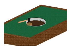
Using a mallet and block of wood tap the top of the edging to position the tree ring firmly into place.
