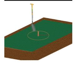
Firstly, mark out where you wish to put the Tree Ring according to the size you have ordered. For 600mm Tree Ring mark a 300mm radius, for a 900mm Tree Ring mark 450mm radius.
