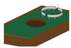
Position the edging sections on a flat even surface, this will be 2 sections for the 600mm and 3 sections for the 900mm. Using the bolts provided secure the edging sections together.
