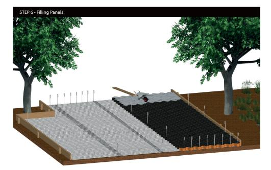
**6.** Starting at one end, begin to fill the cells progressively using CORE SubFlow20 or SubFlow40 clean angular 4/20 - 20/40mm cohesive stone. Limit the drop height to less than 1m to avoid collapsing unfilled cells.
