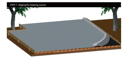
**7.** If the edging you installed in Step 2 is not the correct height or a different edging detail has been specified such as a granite sett or concrete kerb, this can be installed on top of the CORE TRP panel. The concrete haunching can go inside the cells of the TRP panel and on top to create an extremely strong and robust edge.
