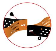
**5.** When connecting ends of adjacent panels align the elongated holes in the centre of the cell walls. Insert the stud through the holes in both panels and attach the securing nut.
