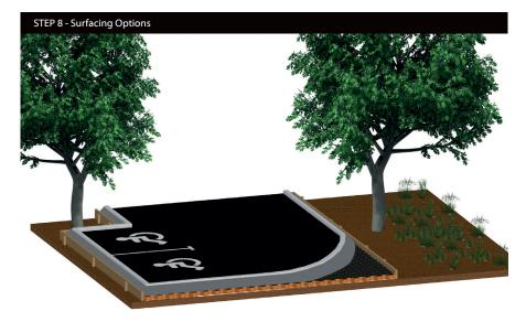
8. The wearing course over the TRP panel must be porous. There are several options including; porous asphalt, permeable block paving; porous gravel or grass grids; resin bound; and rubbercrumb surfacing. For specific construction diagrams please refer to page 11.
