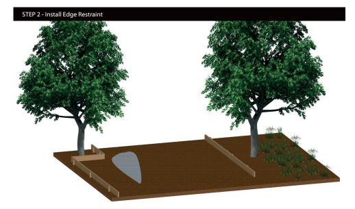
2. An edge restraint should be used around the perimeter of the TRP area. Tanalised timber and railway sleepers are the most commonly used edging for TRP systems. If a more substantial edging is required, concrete kerbs or path edgings can be used. *Edgings for the wearing course are explained in greater deatil in Step 7.*
