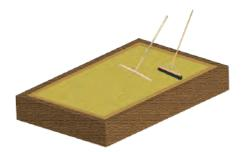
Cover the MOT with a 20-30mm layer of coarse sand or 3-6mm aggregate and level using a wooden spazzle or the back of a broom. It is optional to lay a CORE Shockpad to acheive a more cushioned surface.
