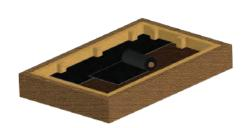
Edge the area with a tanalised wooden batten use small stakes to hold the edging in place and fix with galvanised screws or nails. Cover the area with a geotextile membrane, this will help prevent weed growth and stop the sub-base migrating into the soil below.
