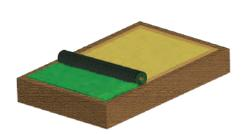
Position the roll at one edge and unroll over the layer of sand, try not to drag the grass into place as this will disturb the levelled layer of sand. Ensure the pile is facing the main viewpoint.
