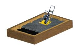
Cover the membrane with MOT type 1 aggregate to a depth of 75mm\* and compact using a vibrating plate or roller to form a suitable sub-base. (75mm or necessary depth to achieve firm ground).
