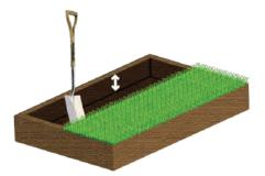
Remove existing turf and excavate to a depth of approximately 100mm and remove any large protruding stones that remain to create a semi-smooth surface.
