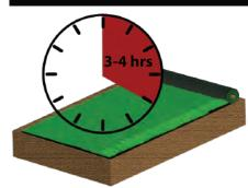
For best results, leave the grass for 3-4 hours or overnight if there are any prominent wrinkles or creases allowing time for them to drop out before trimming and securing.
