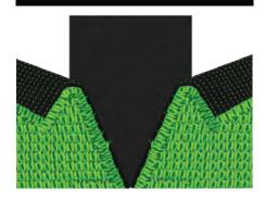
To join the grass ensure the pile is facing the same direction, peal back the two joining edges and lay the seaming tape in the centre of the joint. Ensure to remove the manufacturing strip before joining.
