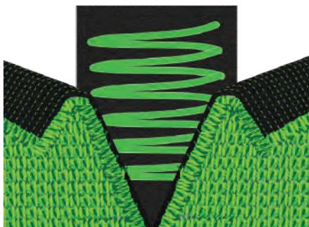
Apply the adhesive to the seaming tape in a zig zag formation. Fold back the two joining edges and press down firmly to form a neat joint.
