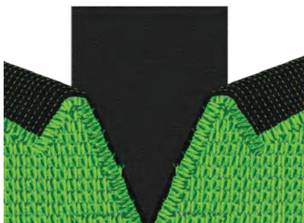
To join the grass ensure the pile is facing the same direction, peel back the two joining edges and lay the seaming tape in the centre of the joint. Ensure to remove the manufacturing strip before joining.
