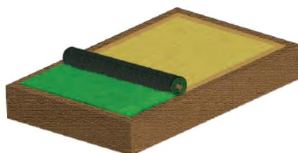
Position the roll at one edge and unroll over the layer of sand, try not to drag the grass into place as this will disturb the levelled layer of sand. Ensure the pile is facing the main viewpoint.
