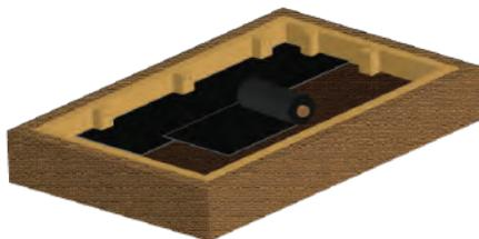
Edge the area with a tanalised wooden batten use small stakes to hold the edging in place and fix with galvanised screws or nails. Cover the area with a geotextile membrane, this will help prevent weed growth and stop the sub-base migrating into the soil below.
