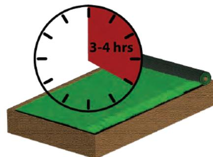
For best results, leave the grass for 3-4 hours or overnight if there are any prominent wrinkles or creases allowing time for them to drop out before trimming and securing.
