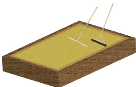
Cover the MOT with a 20-30mm layer of coarse sand or 3-6mm aggregate and level using a wooden spazzle or the back of a broom. It is optional to lay a CORE Shockpad to achieve a more cushioned surface.
