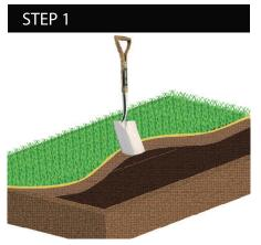
Using a hose or rope, make a guide for for your edging to follow. If the ground is relatively soft you're good to go. If not, you may need to loosen the ground with a flat spade or pickaxe to ensure the edging can be installed without difficulty.
