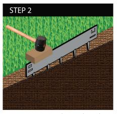
Starting at one end, tap the edging down using a wooden block and mallet. Ensure the edging remains vertical as it is driven into the ground, this prevents twisting when it comes to installing your next edging.
