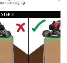
If using the edging on a lawn area the top of the edging should be flush with the soil to prevent the lawn mower blade making contact with the top of the edging. STEP 3
