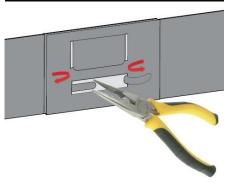
Connect the edgings by sliding the large tab on one edging down through the slit on the adjacent edging. Using a pair of thin nosed pliers, pull both thin tabs through the slit provided and rotate them back on themselves.
